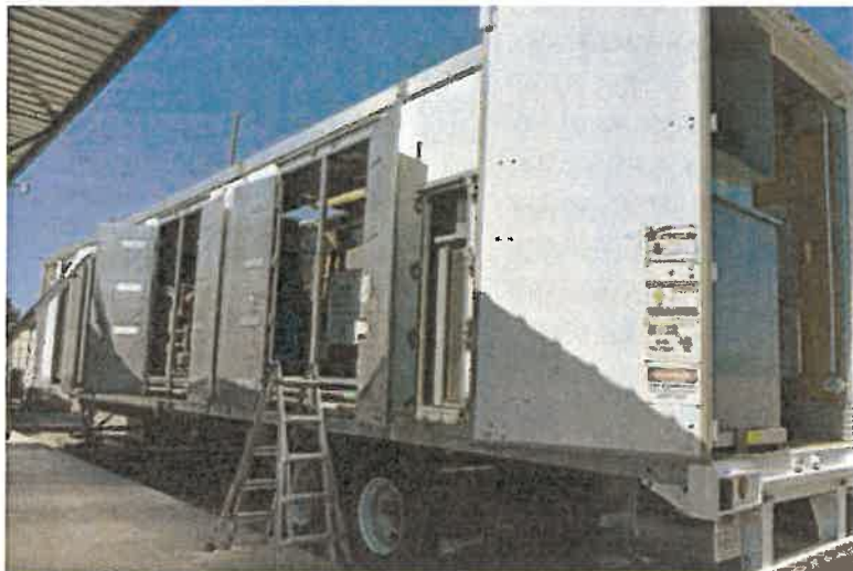
BRE's system also incorporates a microgrid so it can be deployed off-grid in a resort or a village and provide locally produced energy from wastes.
