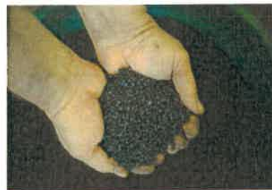
UBQ's process turns unsorted garbage into a bio-based thermoplastic composite. AP
