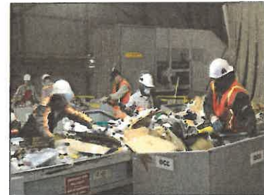
Workers on the platform pull cardboard, paper, plastics & glass and drop them into corresponding bins where the material is collected at the ground level.
