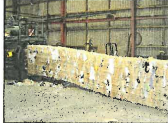
Separated materials are compacted into bales and are ready for end markets. Manufacturers purchase the commodities and make them into other plastic, paper, glass, and metal products.
