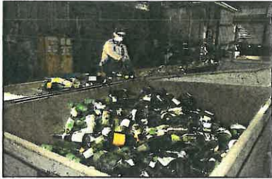
Glass is sorted by color. Plastics are separated by type. Paper is separated by grade (mixed paper, white paper, newspaper, cardboard, etc.). Steel & Aluminum are captured by magnets and air currents.
