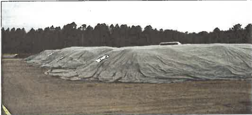
Compostable material is ground into small pieces and formed into piles. The piles are covered with a breathable fabric that accelerates the natural cycle of decomposition with higher temperatures.
