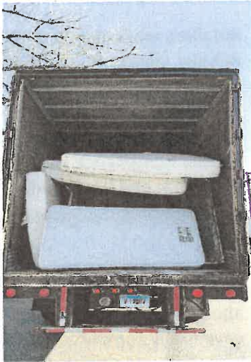
Improper Stacking Method This load would be rejected at recycling facilities.
